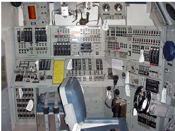
TYPICAL SSN/SSBN BALLAST CONTROL PANEL
