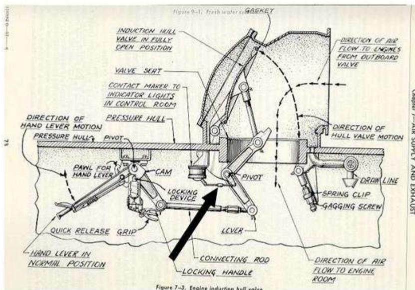
What would happen if the Contact Maker Linkage on a Sargo class diesel boat was not connected to the Engine Induction Hull Valve Pivot? Simply put, the Christmas Tree would show the Induction Valve shut when it actually was open! And this is exactly what caused the loss of Squalus, according to TMC(SS) Ret. Arthur Dawes in an interview that I conducted with him in the early 1990s.
