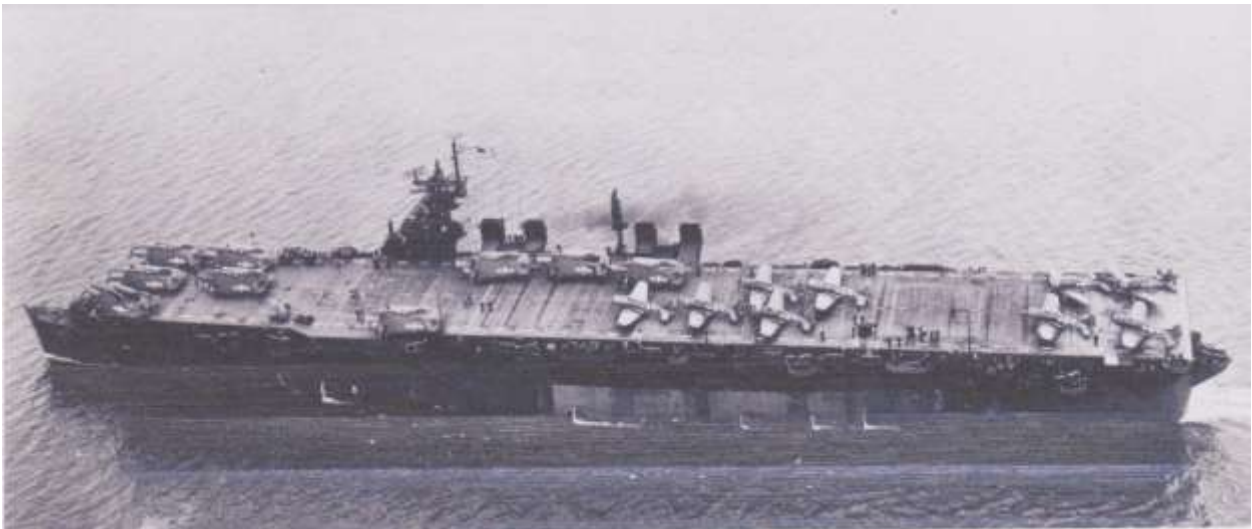
The USS Independence during a better time. She was used in the atomic bomb test and after testing later sank off the California coast. Note that the hull was intended for a cruiser.
